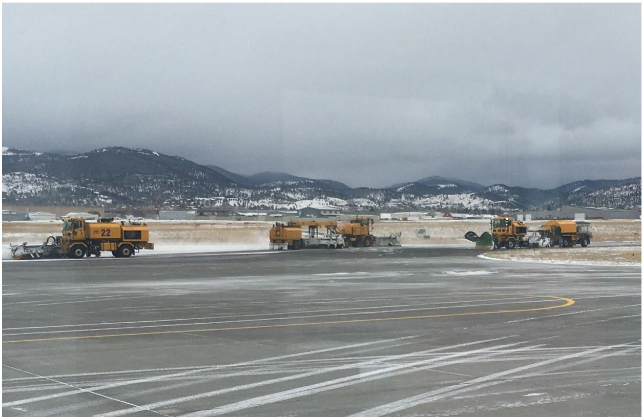
Newer Equipment - 2 Combo Plow/Brooms / Front Mount Sweeper
